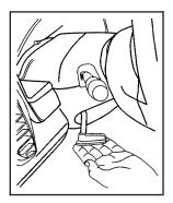
The lever that allows you to tilt the steering wheel is located on the left side of the steering column.
